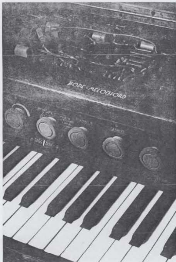
3. Part of the front panel of Bode's first Melochord (1947). Akademie der Künste, Berlin, Werner-Meyer-Eppler-Archiv, Nr. 278.
