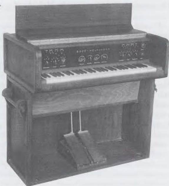
2. Large Melochord model with 5 octave keyboard in an advertising photo, Akademie der Künste, Berlin, Werner-Meyer-Eppler-Archiv, Nr. 278.
